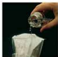
2. POUR SAMPLE/ COLILERT MIXTURE INTO QUANTI-TRAY.
